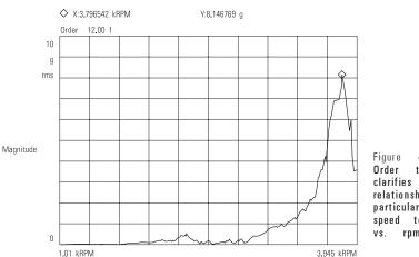
Figure 4: Order tracking clarifies the relationship of a particular shaft speed to amplitude vs. rpm.
