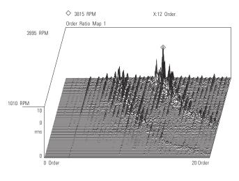
Figure 3: An order map clarifies the relationships between shaft speed and vibration amplitude.
